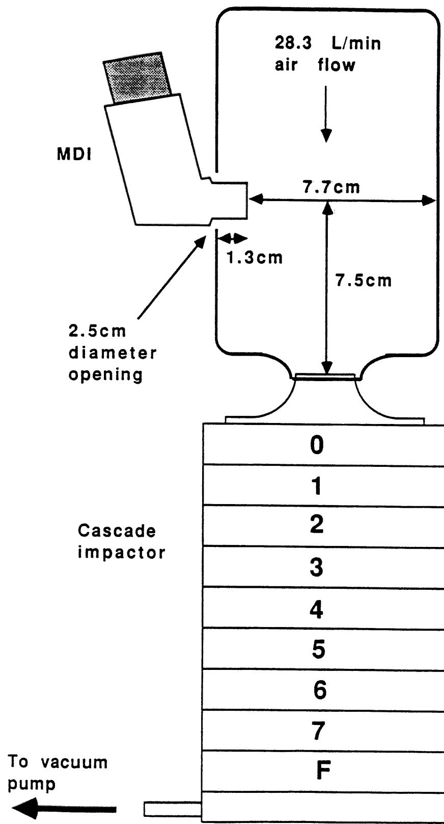
**FIGURE 2 : DEPOSITION STUDY WITH SPACER**
